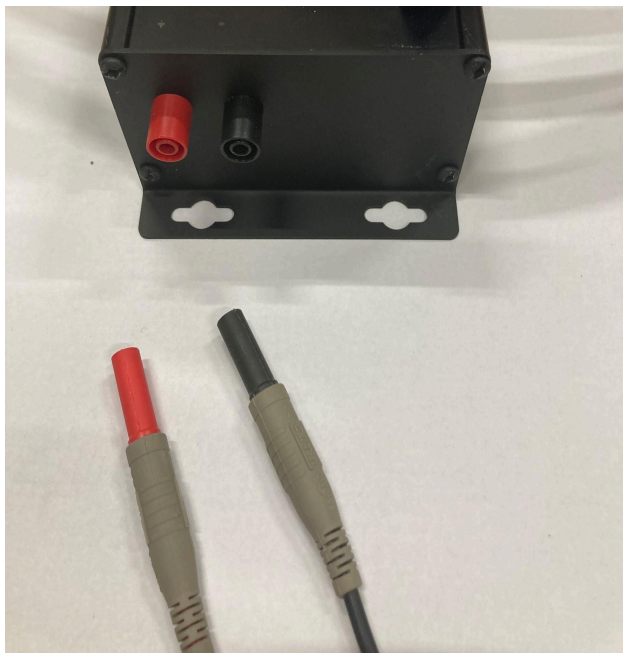
Fig 5.1.2: Connect the banana connector to the EMU
