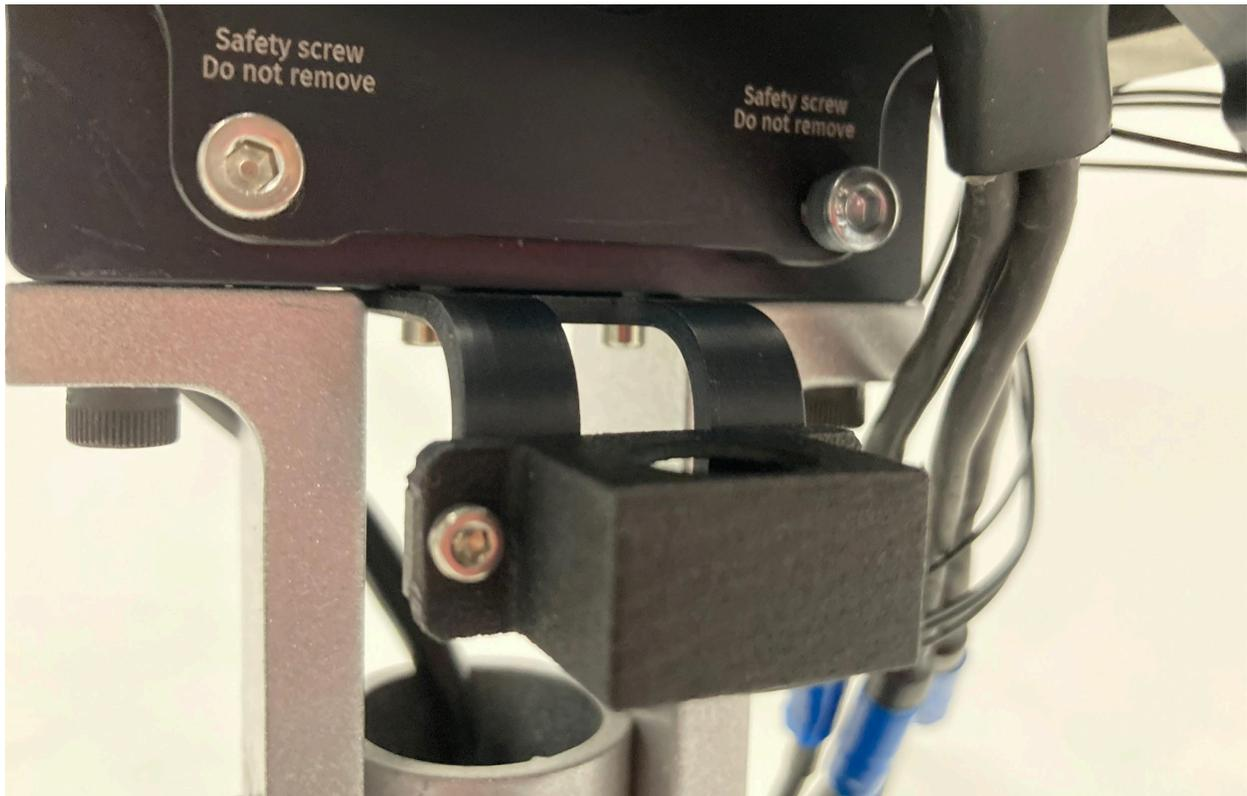
Fig. 10. Installation of the assembly on the FMU
