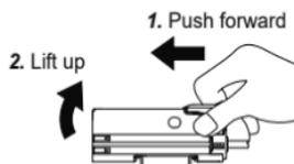
Fig. 17. Mount the amplifier on a DIN rail
