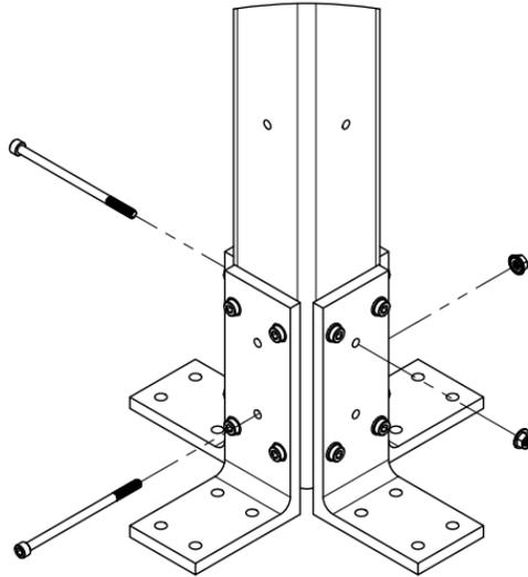
Fig. 2. Stand Assembly - Lower Section with Reinforcement Bolts
