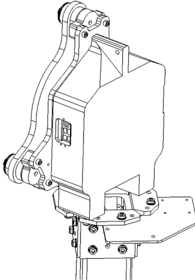
Fig. 29. Install the support plate with the sensors facing downward
