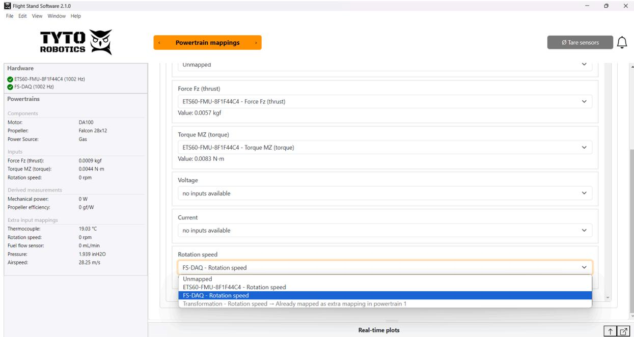
Fig. 53. Hardware mapping of the RPM sensor
