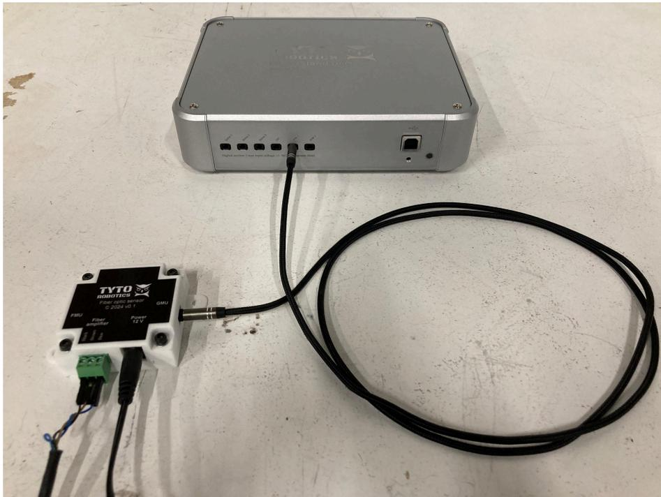
Fig. 22. Connection of the audio jack cable between the DAQ and the converter
