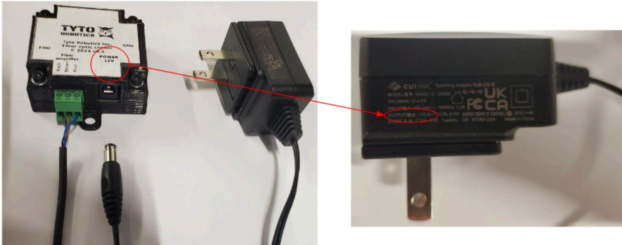
Fig. 21. Connection of the **12 V** power supply to the signal conditioning unit
