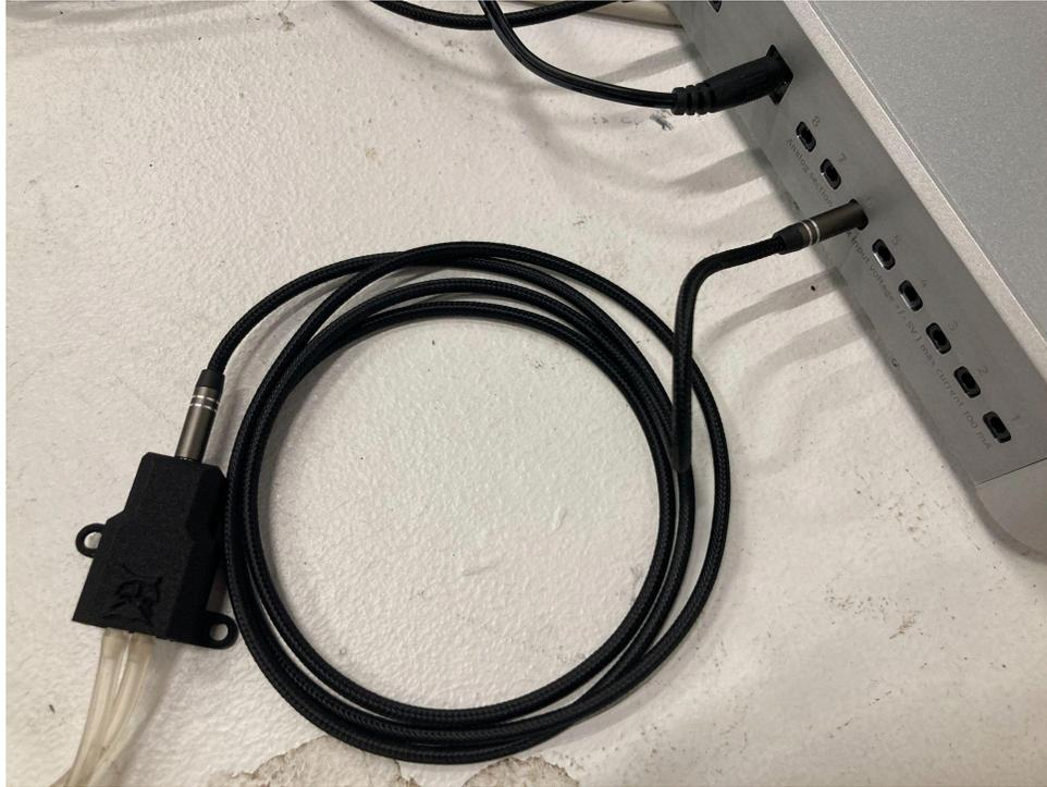
Fig. 37. Connections of the pitot tube, pressure sensor, and the DAQ
