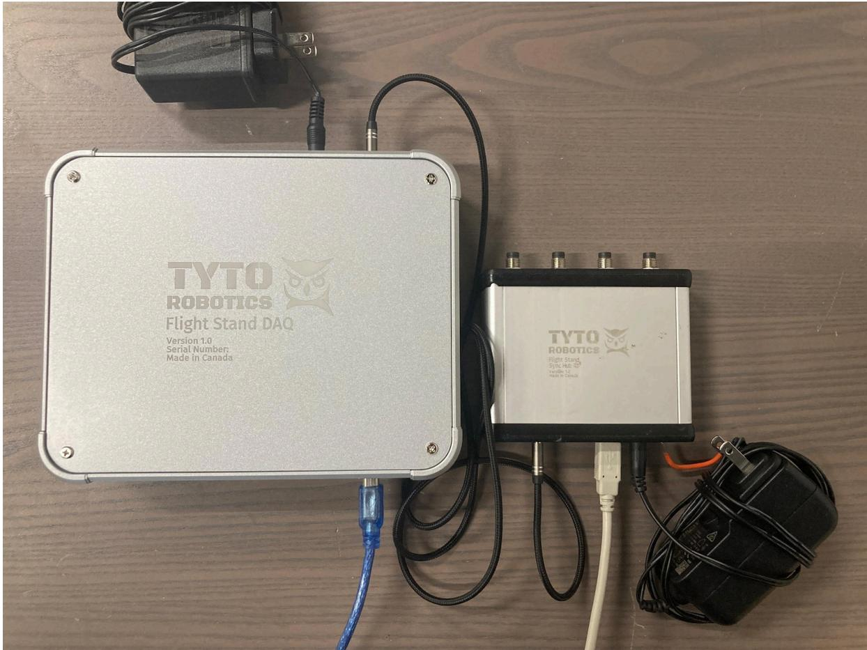
Fig. 38. Sync Hub and DAQ connections with sync cable (IN to OUT), and each device's power source, plus USB connection to the PC
