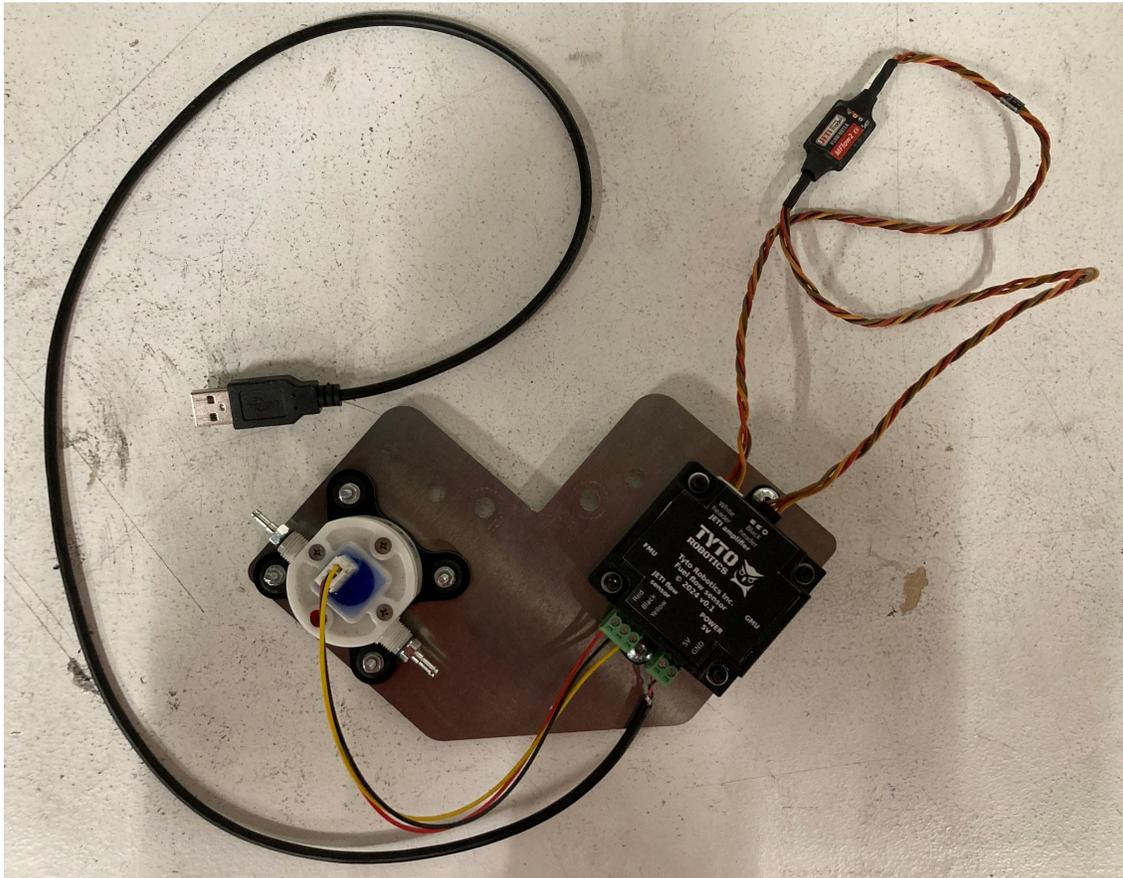
Fig. 28. Fuel flow sensor and converter unit fully installed and connected on the support plate
