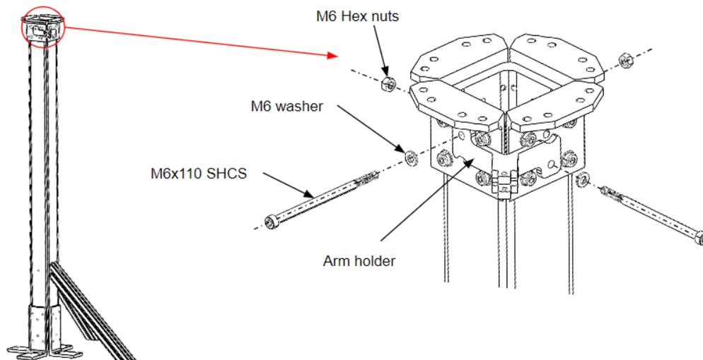
Fig. 10. Fiber arm holder on the Flight Stand 60 / 150
