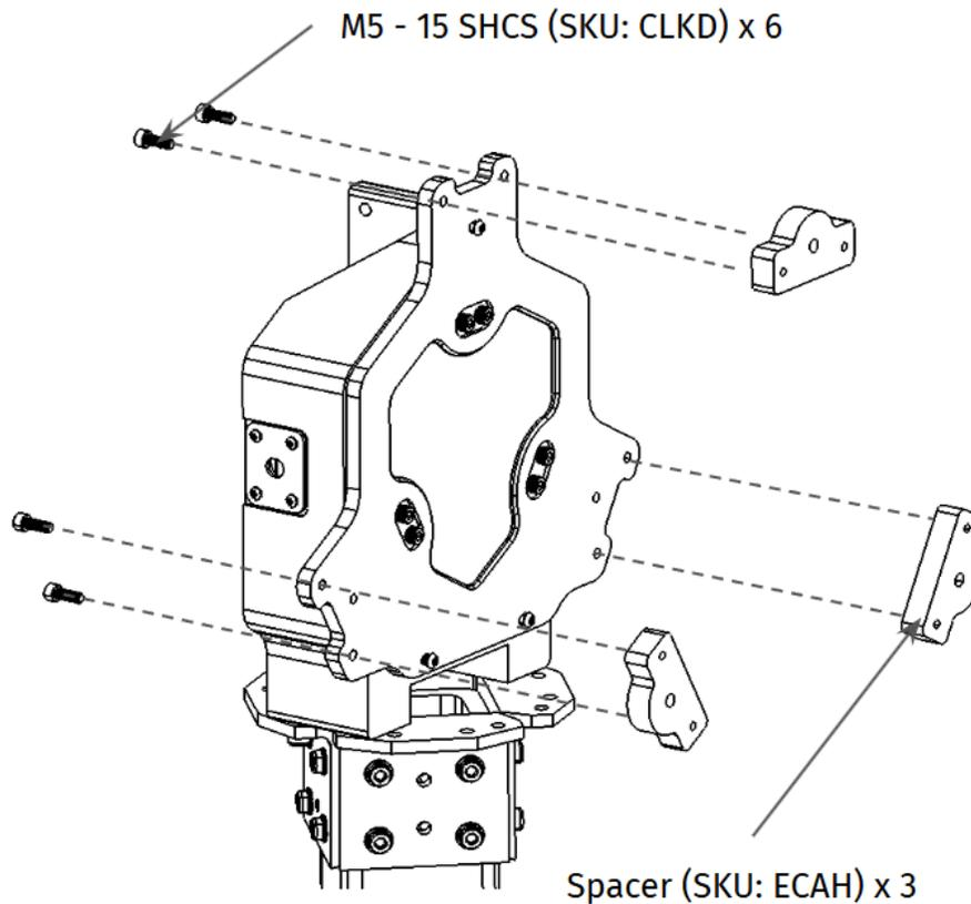
Fig. 7. Install spacers on the FMU
