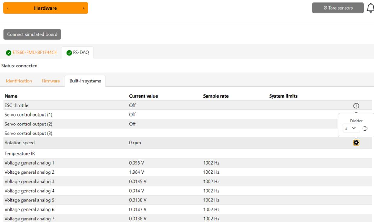
Fig. 54. Divider setting in the Flight Stand software
