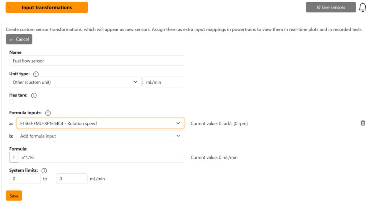
Fig. 56. Input transformation for flow rate reading
