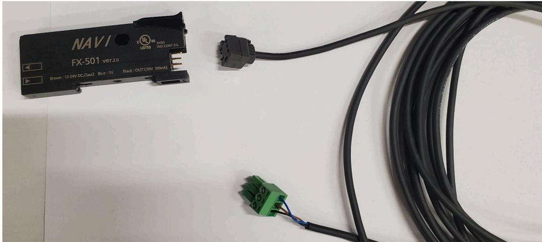
Fig. 19. Connection of the electrical wire to the amplifier
