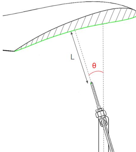
Fig. 13. Fiber optic sensor's position on the Flight Stand 60 / 150
