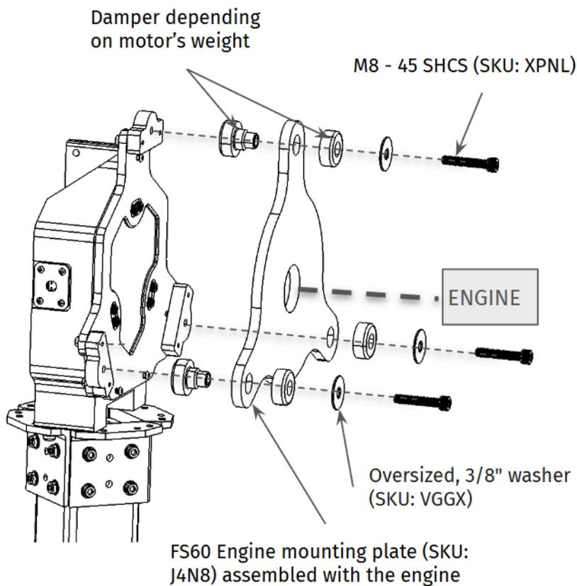
Fig. 9. Mount the engine mount with engine and vibration dampers
