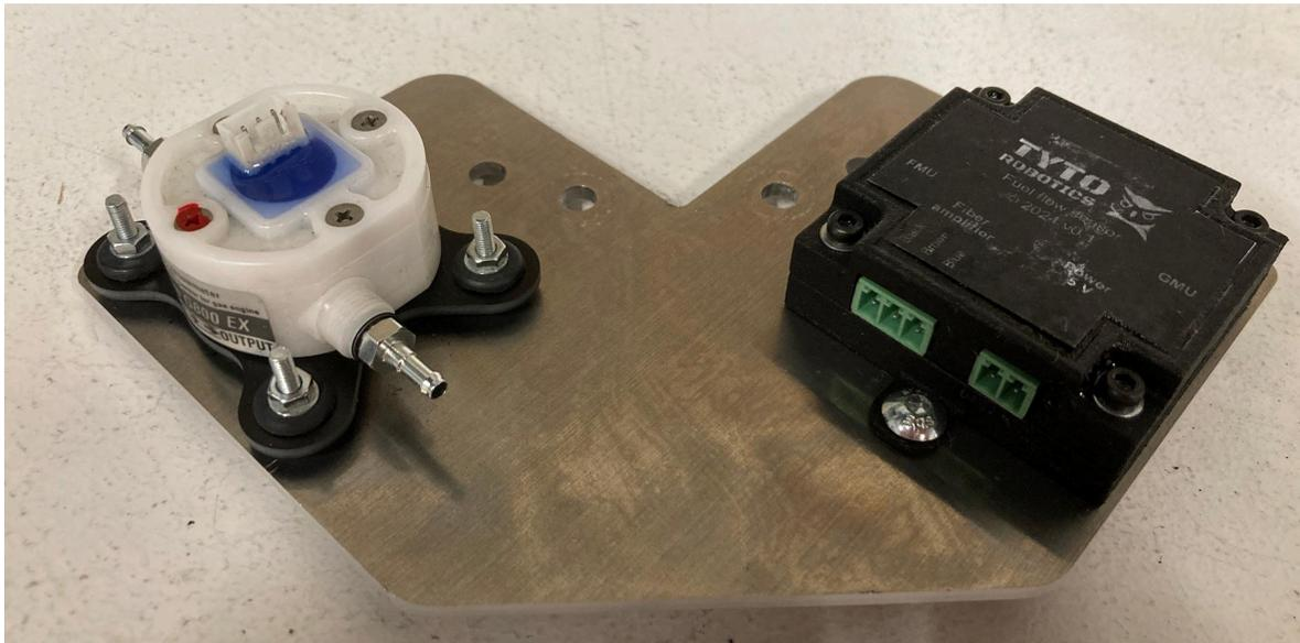
Fig. 25. Support plate with fuel flow sensor and fuel flow converter unit
