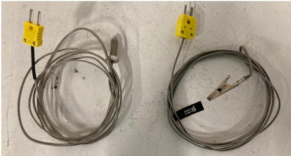
Fig. 35. Different K type thermocouples
