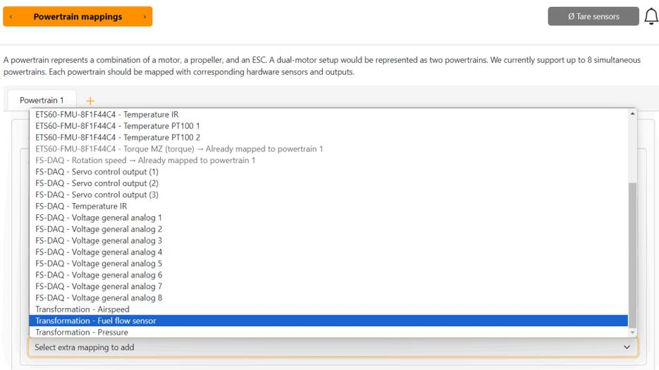
Fig. 57. Extra mapping of Fuel flow sensor in the software
