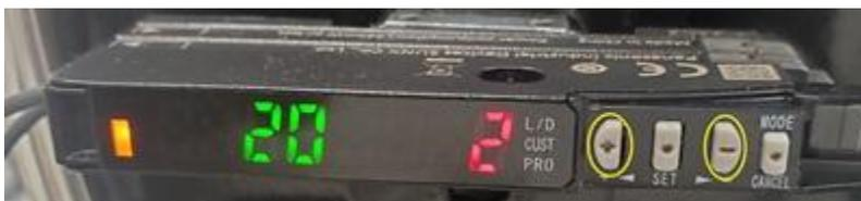
Fig. 52. Setting of the threshold
