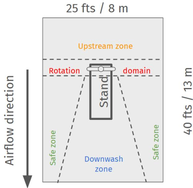
Fig. 39. Safe zone for the work station at your facility
