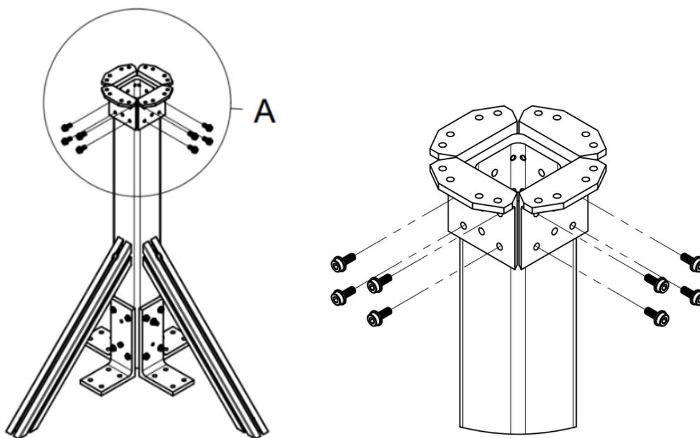
Fig. 4. Stand Assembly - Upper Section with four L-Brackets
