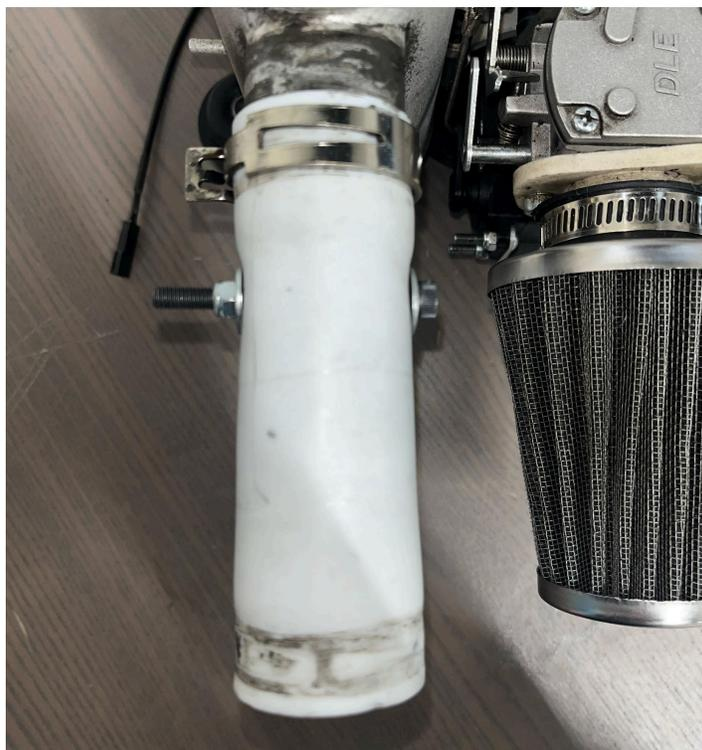
Fig. 32. A bolt that passes through the exhaust with lock nut
