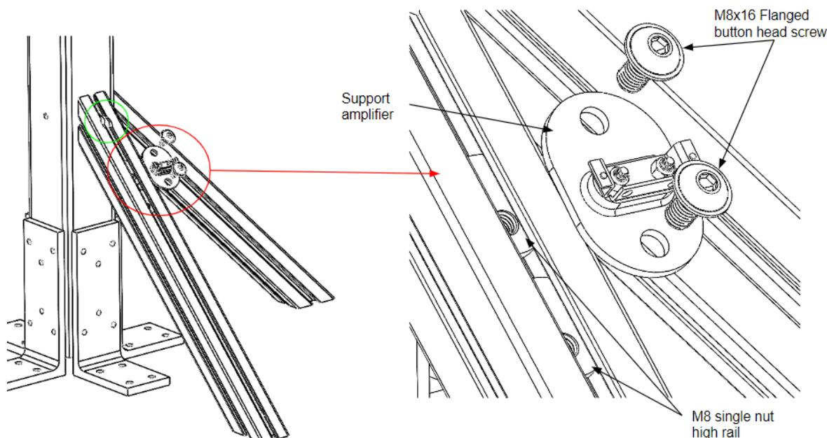
Fig. 16. Support amplifier on the Flight Stand 60 / 150
