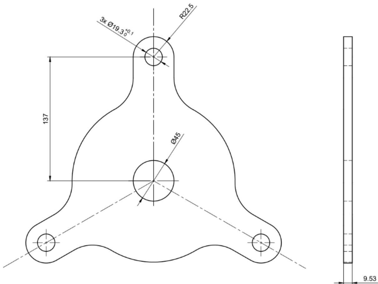
Fig. 8. Engine mounting plate
