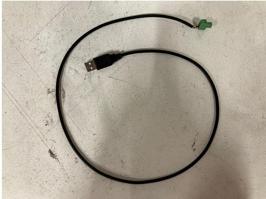
Fig. 26. USB cable with 5V and GND to the fuel flow converter unit
