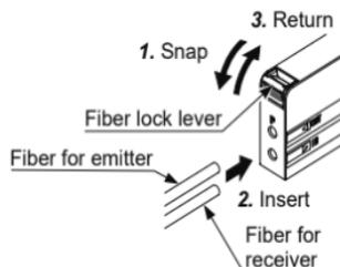
Fig. 18. Connect the fiber cables on the amplifier
