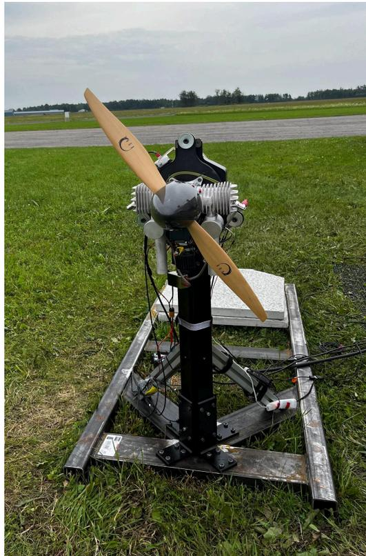
Fig. 5. Ground base for engine test stand
