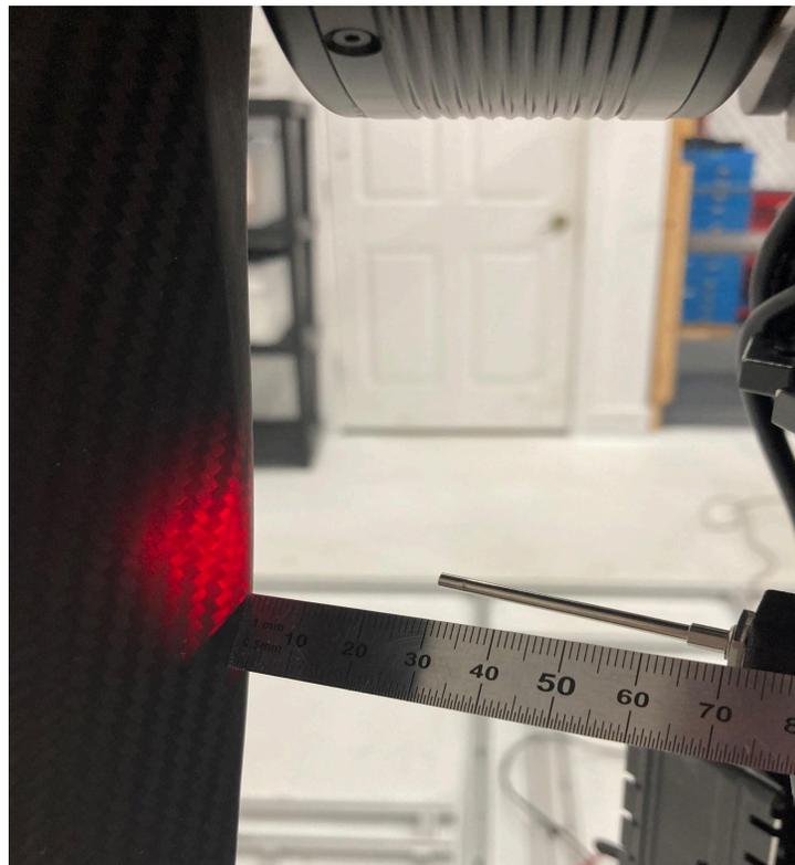
Fig. 14. Fiber head at around 30 mm from the prop at the closest
