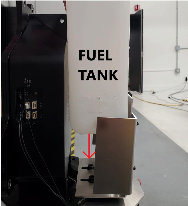
Fig. 63. Example of placing the fuel tank behind the FMU
