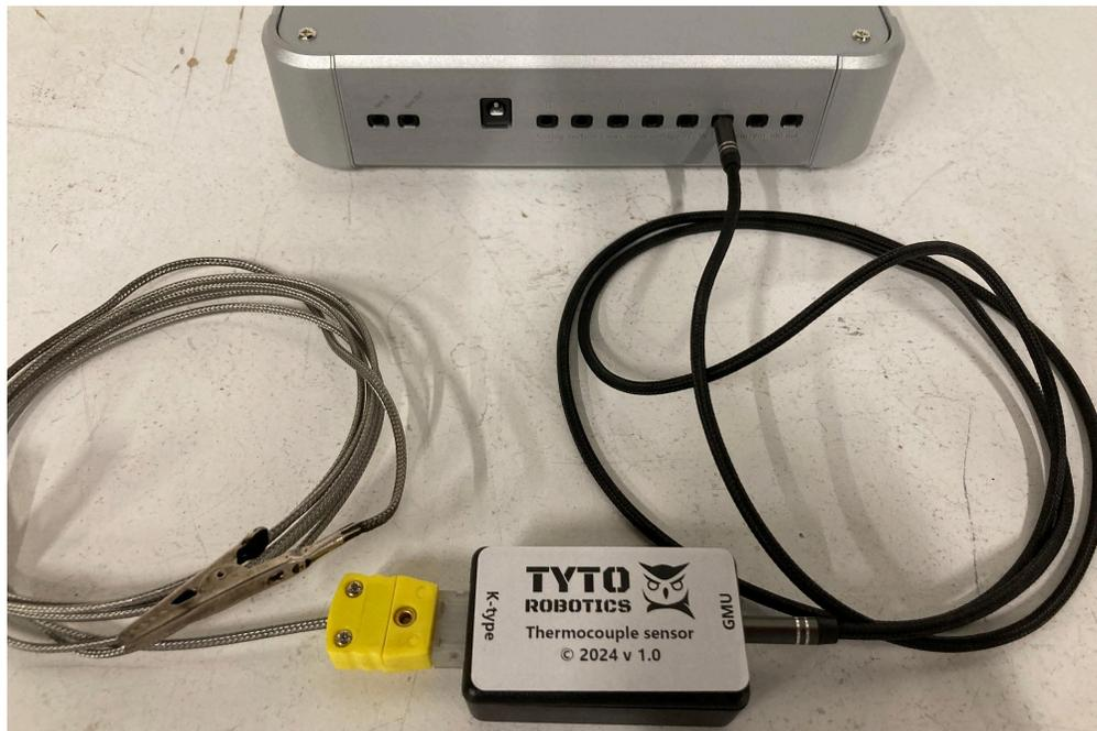
Fig. 34. Connect the thermocouple breakout to any analog port on the DAQ
