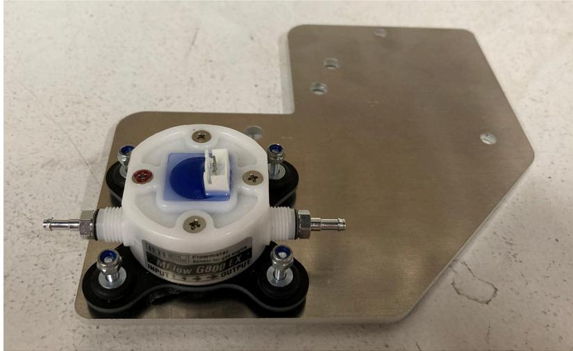
Fig. 24. Fuel flow sensor on the plate, inlet on the left, and outlet on the right
