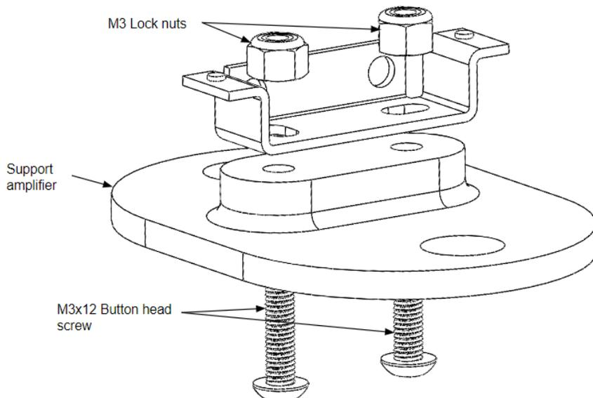
Fig. 15. Assembly of the support amplifier for the Flight Stand 60 / 150
