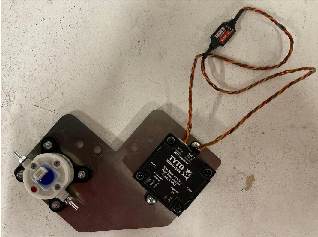
Fig. 27. Jeti amplifier interconnects on the fuel flow converter unit [B: Brown, R: Red, O: Orange]
