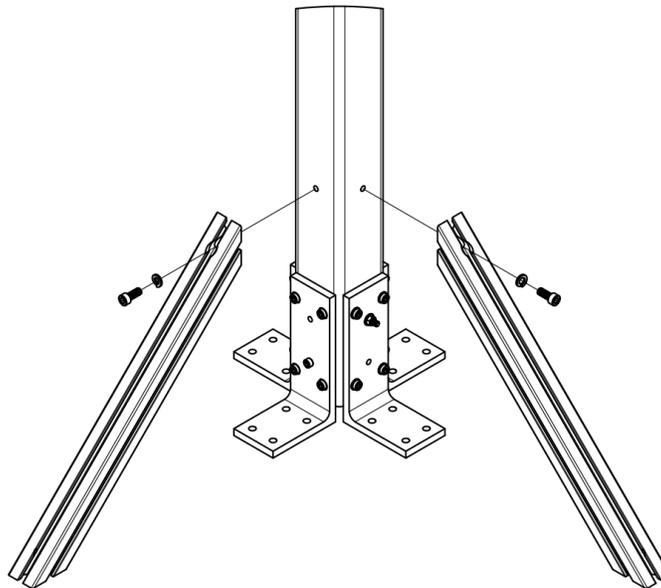
Fig. 3. Stand Assembly - Lower Section with 45-Degree Support Beams
