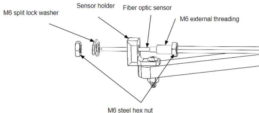
Fig. 12. Fiber optic sensor on the sensor holder on the Flight Stand 60 / 150
