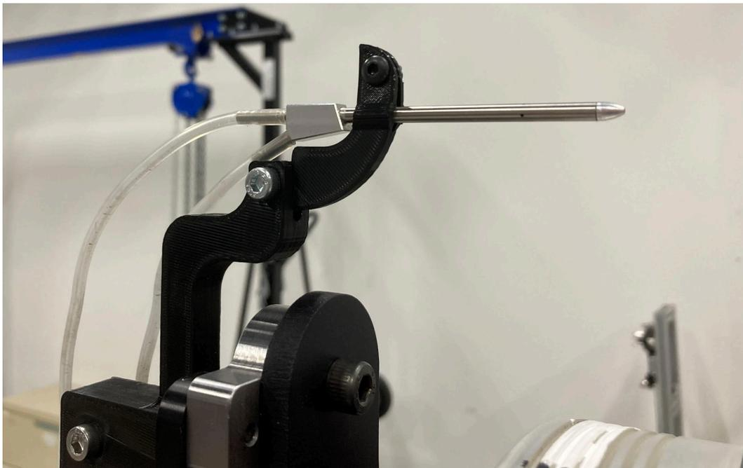
Fig. 36. Example of pitot tube and its fixture (yours to prepare)
