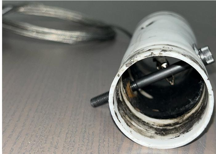
Fig. 33. Alligator clip thermocouple clipping on the bolt inside the exhaust
