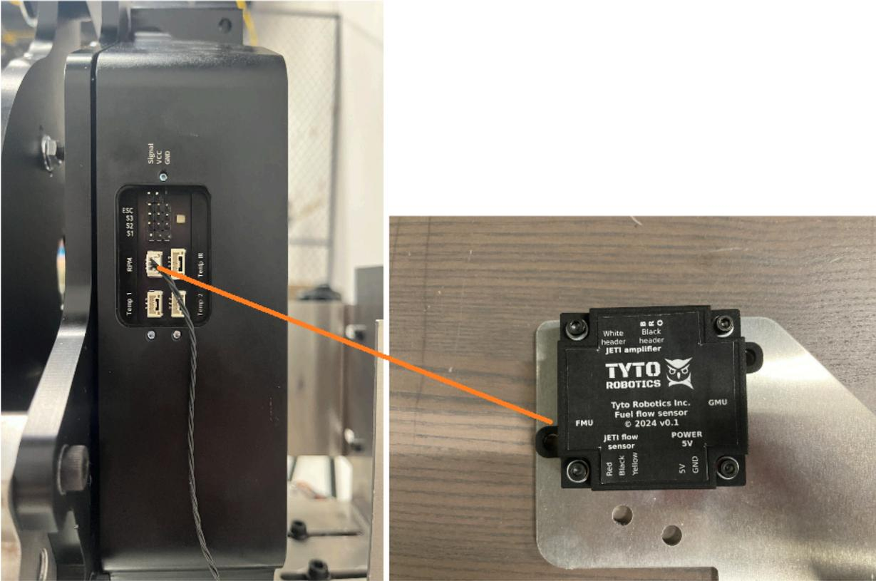
Fig. 30. Plug the 3-POS JST wire from the fuel flow converter to the FMU's RPM port
