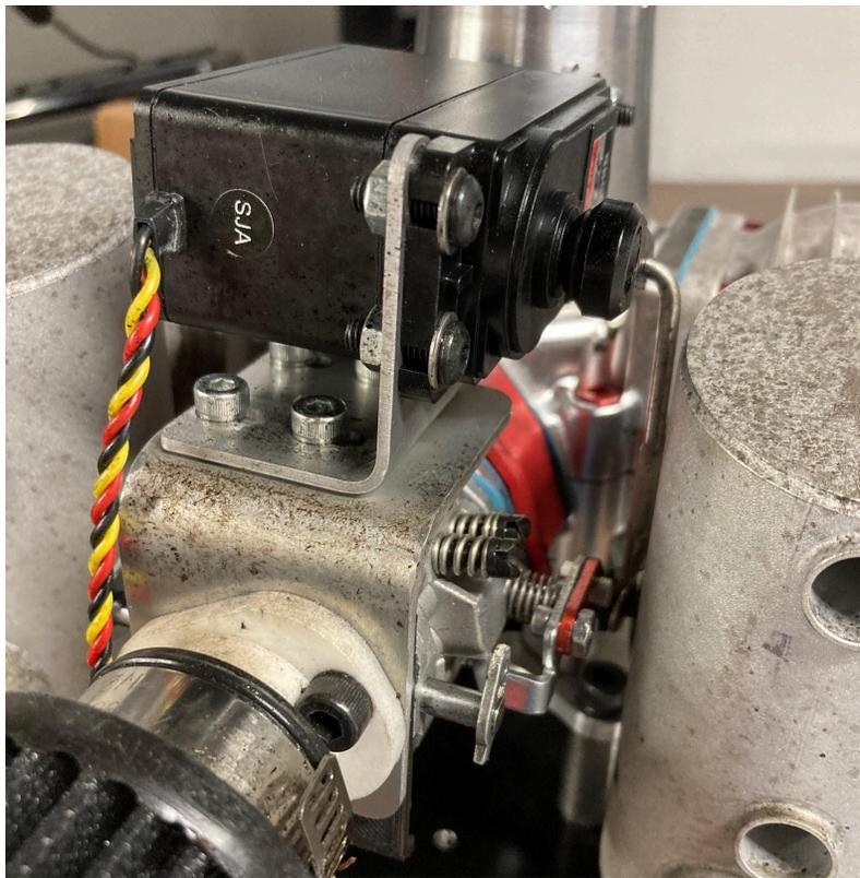
Fig. 62. Example of throttle control mechanism (yours to prepare)
