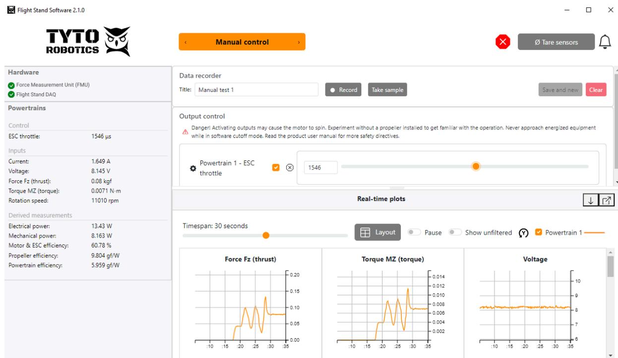
Fig. 65. Flight Stand software throttle slider in the Manual Control tab
